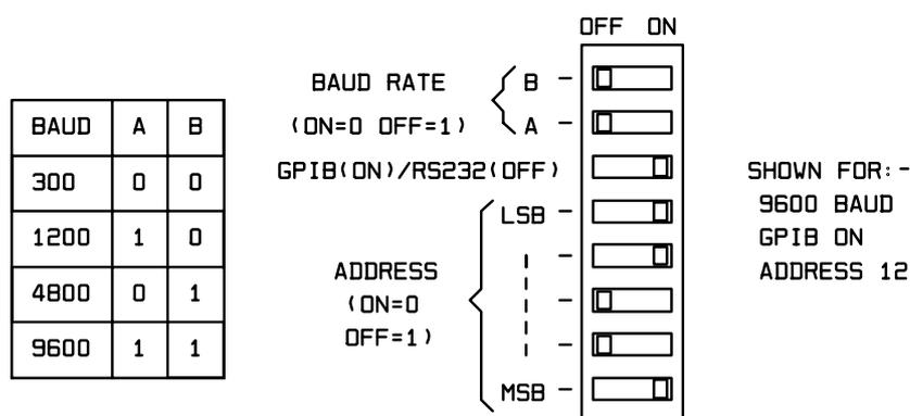
Most switch states are read at power up so changes may not be acted upon if the instrument is already powered on and it will be necessary to switch off then on again to make the settings valid.
