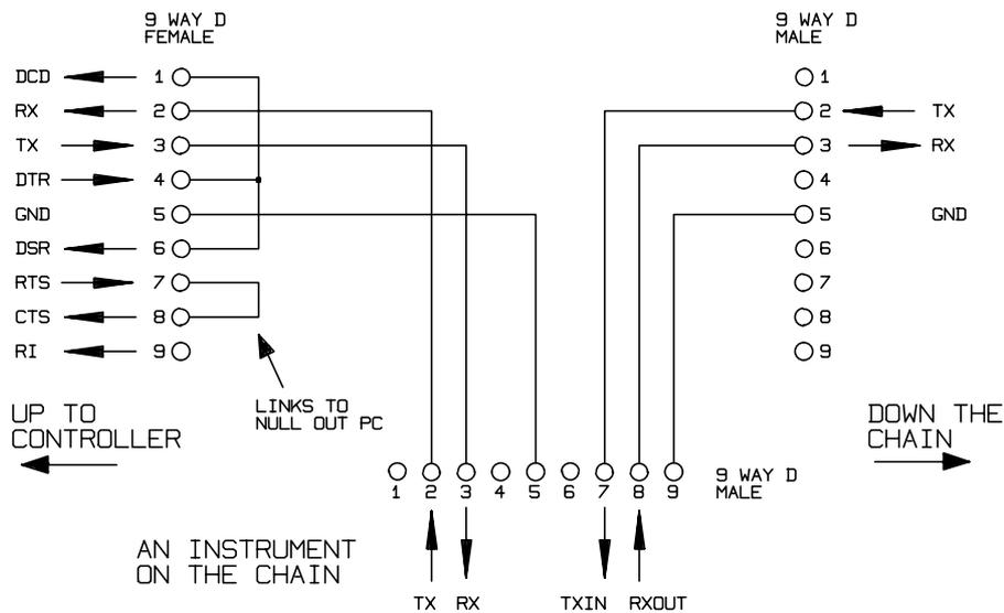
All instruments on the interface must be set to the same baud rate and all must be powered on, otherwise instruments further down the daisy chain will not receive any data or commands.
