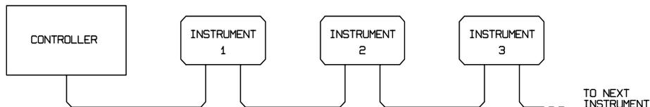
The daisy chain consists of the transmit data (TXD), receive date (RXD) and signal ground lines only. There are no control/handshake lines. This makes XON/XOFF protocol essential and allows the inter-connection between instruments to contain just 3 wires. The wiring of the adaptor cable is shown below:
